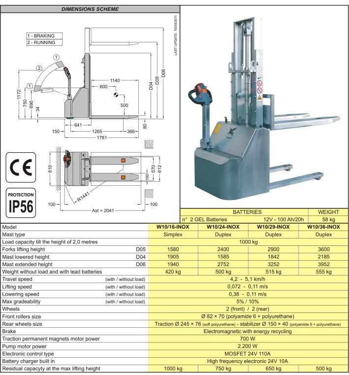
The WID INDX stackers series are designed to be the most compact, handy and easy to use for every user. The mast is extremely compact in height to allow to pass also under very low doors and the narrow stearing radius together to the compactness of the machine body in depth permit to move with agility in all the narrow spaces. The lateral tiller and the compactness of the machine body also in width and in height allow a large visibility and handy in all the manoeuvres.
