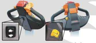
Roller to control the lifting + descending speed of the forks
